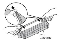
The toner cartridge is installed correctly when the triangles match.
